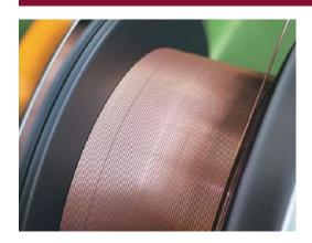
Within FCAW (Flux Cored Arc Welding), seamless cored wires offer optimal protection against moisture reabsorption. During use, moisture cannot penetrate into the filling since there is no closed seam running over the wire length. This extremely low level of diffusible hydrogen prevents the weld from hydrogen induced cracking or cold cracking.
