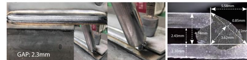
[ 590MPa Zinc Coating Steel 2.3mmt LAP JOINT, Ar+CO<sub>2</sub> (9:1), 180A/16V ]
